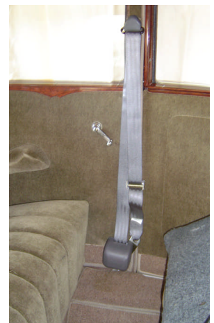
Figure 5 Driver's Seat Belt showing retractor installation
