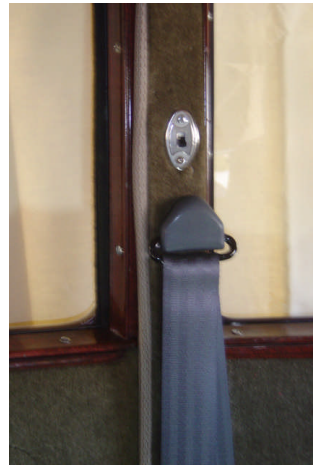
Figure 4 Passenger's Seat Belt mounted under light switch
