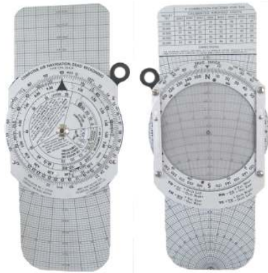
Front and back sides of a modern version of the Dalton E-6B Aerial Navigation Computer
