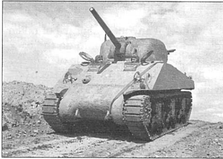
Sherman M4A3 medium tank powered by modified Ford 12 cylinder airplane engine that became the standard US tank engine
