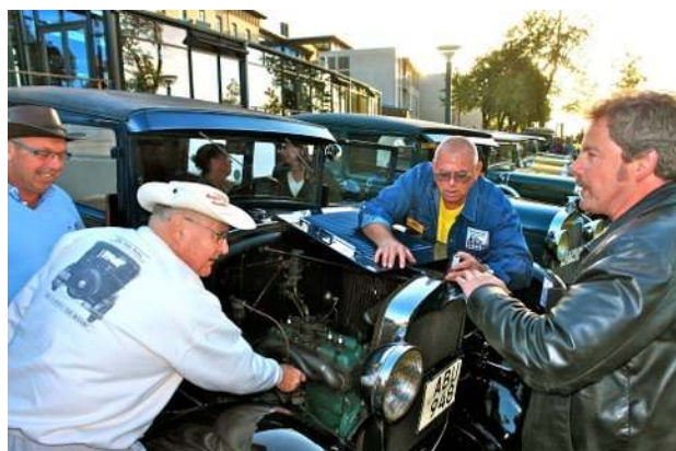
Bob uses his keen ear and nimble fingers to finely tune the carburetor for slow idle
